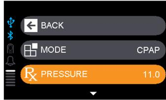
2. Turn knob to Pressure setting and press (set pressure will begin to blink). (Initial Setting = 8) (Default = 10)
