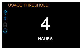
**NOTE** - The SmartCode feature tracks the number of days that the device was used greater than or equal to "usage threshold" hours.
