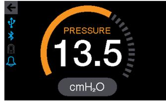
4. Choose Pressure Unit and Press to toggle between options (cmH2O, hPa, mBar). (Initial Setting = cmH2O)
