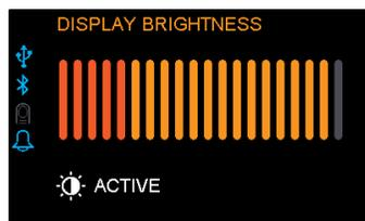
4. Turn knob to select desired Brightness for either Active or Standby for Display or Controls. **NOTE** - Setting adjustable by patient.
