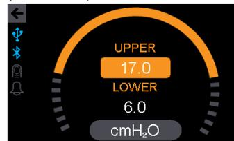
3. Turn knob to Lower and press (set pressure will begin to blink). Adjust then Press to Set. (Default = 7)
