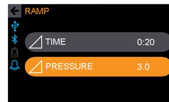
5. Turn Knob to desired Ramp Pressure and Press to Set. **NOTE** - Patient cannot adjust pressure. (Default = 4)
